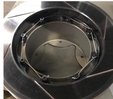
Figure 2 - Properly installed safety wire
