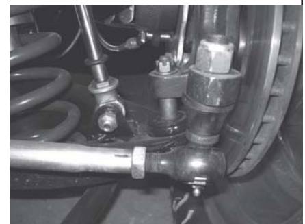
Howe #23284 EZ Bump tie rod end with spacer installed.
